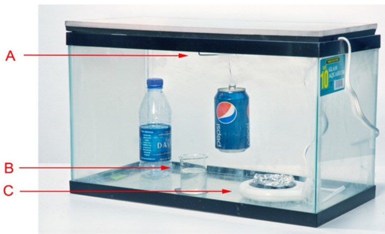
Fig. 11-2 Example of a typical superglue fuming chamber. (A) is a piece of wire from which items can be suspended. (B) is a beaker of hot water. (C) is a mug warmer to heat liquid superglue on a piece of foil.
