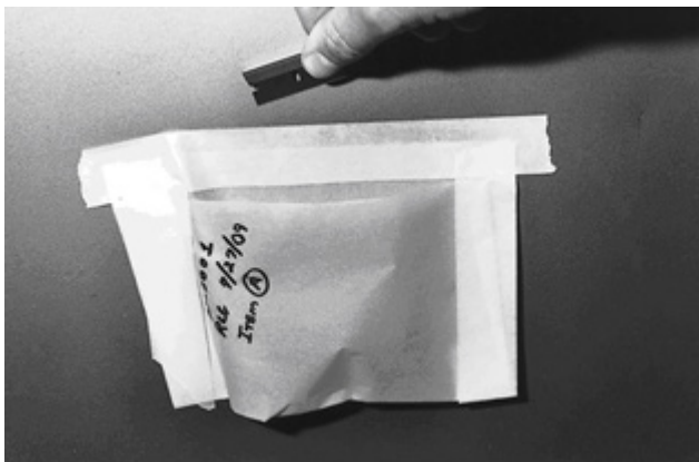
Fig. 17-3 Recovery of Paint Sample: Tape a clean sheet of paper (do not use envelopes) to the object in the manner shown, forming a pocket. Mark the paper for identification. Scrape the questioned paint into the pocket formed by the paper. It is important to use a new, disposable scalpel blade or razor blade for each sample to avoid contamination. Some razor blades are coated with oil to prevent rusting. Therefore, all razor blades should be thoroughly cleaned with a clean cloth or tissue just before they are used.
