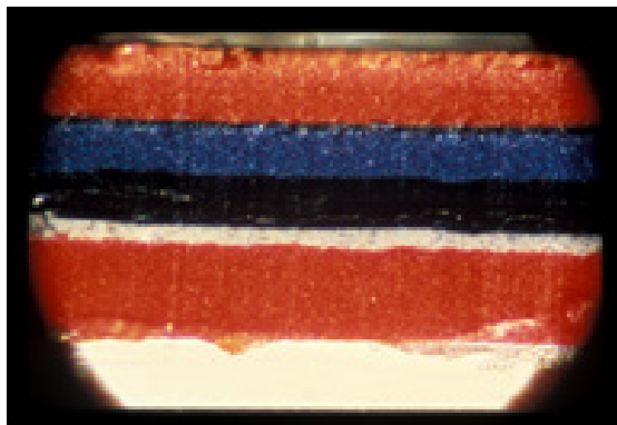
Fig. 17-2 Cross section of multi-layer paint chip. Each layer represents a separate painting operation (Magnification approximately X350).
